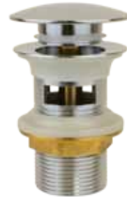
#19007 Pop-Up Drain with overflow for Rectangle Ceramic Sink Material: Chrome Plated Brass Outlet Connection: 1-1/4" Shipping Weight: 1 lbs.
